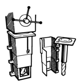
• Shut off power before removing the drill bit.
